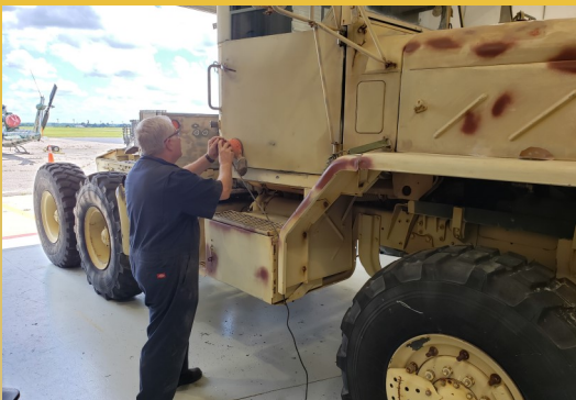
Mark Inabinet working on the surface rust
